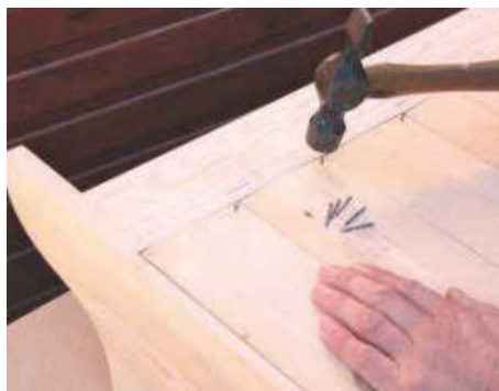
STEP 15. Lay out the matchboard and cut both outer pieces to width if necessary. Pre-drill nail holes to prevent splitting
